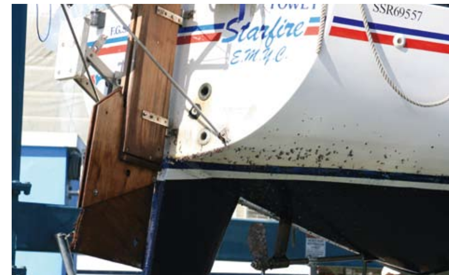
Left: An emotional moment as Starfire reaches St Lucia with jury rudder number three! Above: Granny's shelves and two bunk bases - all you need for a good rudder. Below left: Fresh fruit from a welcoming local boat, a familiar sight in Rodney Bay. Below right: St Lucia never stints on celebration parties
